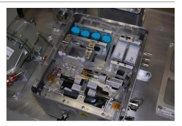
This IntraVenous Fluid Generation (IVGEN) system produces IV-grade water from space station drinking water.
